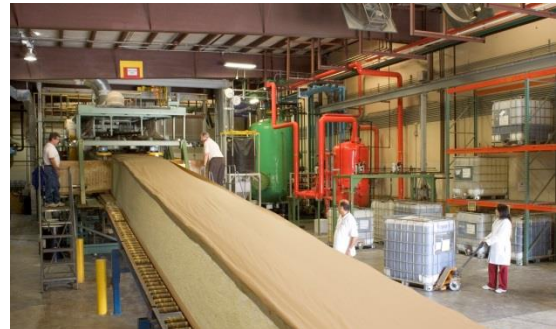
Figure 1: Polyiso exiting the tunnel
