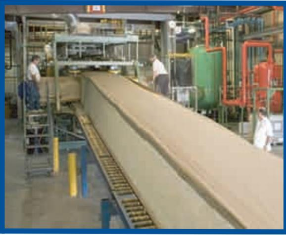
Dyplast Products' polyisocyanurate bunstock exiting the free-rise tunnel. ISO-C1 can then be cut virtually to any length and subsequently cut in sheets to 1/32" tolerance.
